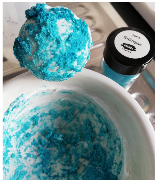
#44450 Verdigris and #75305 Dispersion K 19 form a lumpy mass that is unusable.
