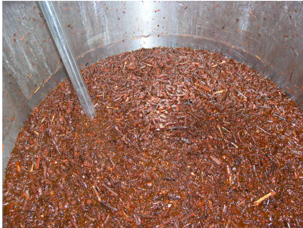
The shredded and washed madder roots are boiled in an alum solution...
